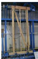
Figure 4: Frame with single brace specimen
