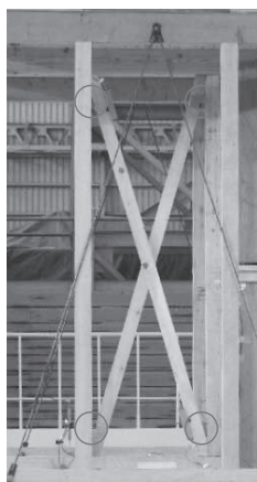
Picture 1: Wood brace fastened by the new fastener
