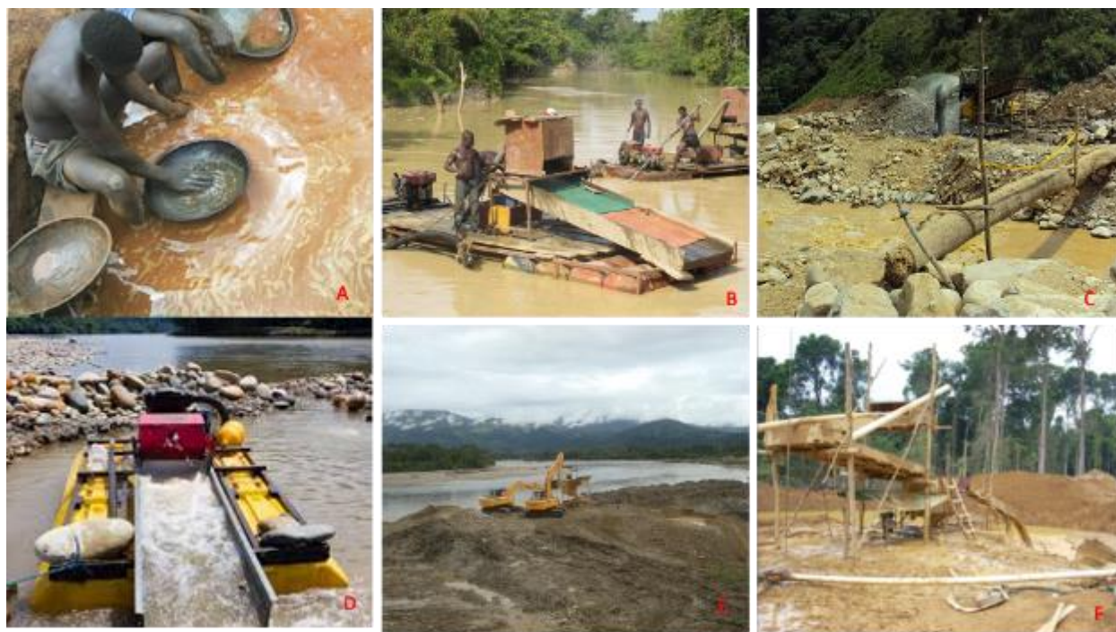
Figure 3. Different modes of work in alluvial and colluvial ASGM. A) panning in the river, Tanzania (B) single sluice box, Ghana (Hausermann et al., 2020) C) single sluice box in Ecuador D) dredge, Ecuador E) Zig Zag sluice box in Ecuador, F) Zig Zag sluice box in Guyana.
