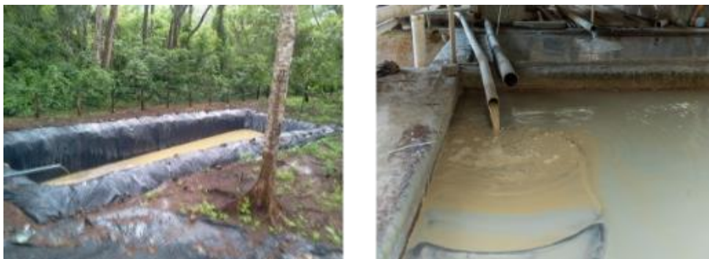
Figure 24. A) an artisanal tailings pond covered with liner at the base to prevent leakage. B) Tailings disposal in cement ponds.
