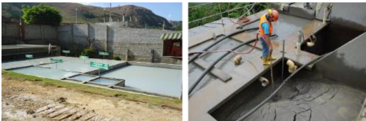
Figure 25. Concrete tailings ponds to separate solids from liquids. The system also facilitates the separation of different types of tailings. The tailings are drained into ponds to settle the solids allowing the liquid to pass through.
