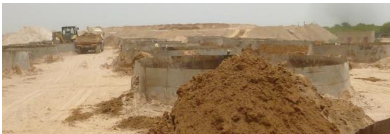
Figure 17. The vat leaching systems using trucks to transport tailings in Burkina Faso (Photo PACT). In these systems, the process of cyanidation lasts for about 20 to 40 days.
