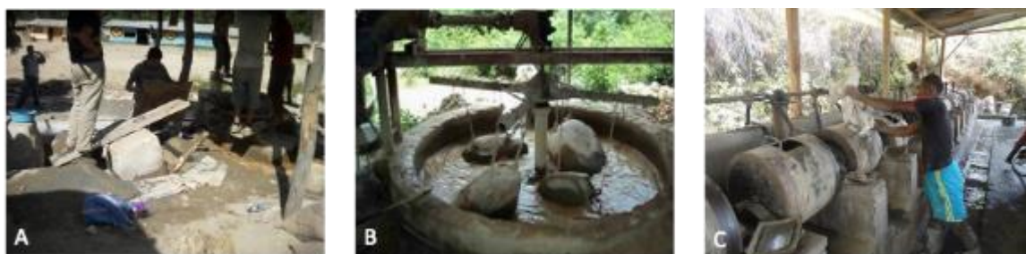
Figure 5. A) The "quimbaletes" Peru B) "Rastras" Nicaragua and Honduras C) "Cocos" Colombia; used to crush and mill the ore and proceed to amalgamation for gold recovery.
