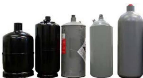
Figure 16. Examples of the mercury containers for temporal storage. Source: UNEP, 2019.
