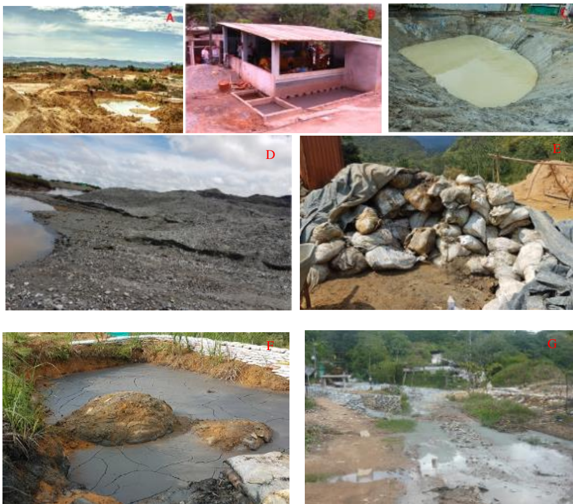
Figure 21. Examples of storage solutions of mercury-contaminated tailings in ASGM: A) deposition in open area, B) deposition in separated holding tanks, C) deposition in earthen tailings ponds, D) tailings accumulated in piles; E) tailings piled in sacks, F) tailings deposited in inadequate tailings ponds, G) tailings scattered in the environment. Source (D-G Pictures): Pure Earth – 2021b.
