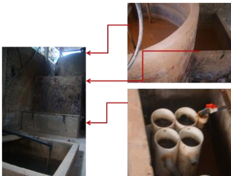
Figure 17. The vat leaching systems using trucks to transport tailings in Burkina Faso (Photo PACT). In these systems, the process of cyanidation lasts for about 20 to 40 days.
