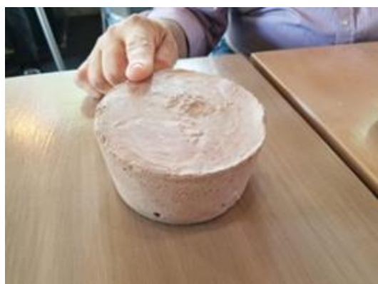
Figure 12. Mercury solidification with cement and sulfur in Costa Rica. (source: Marcello Veiga)
