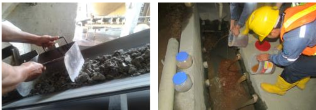
Figure 8. Sampling the head ore at the milling process entrance in a Chilean mill (right) and sampling the slurry at the discharge of the mill (left). The team must follow the miner's procedures and adapt the sampling according to each ASGM site's operational mode.
