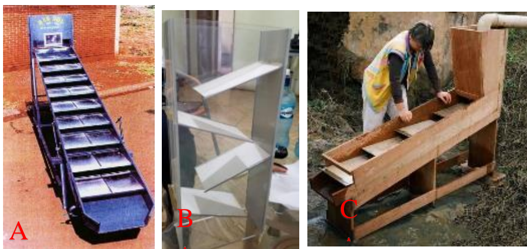
Figure 11. Various design model of the metal coated plates to remove mercury from tailings. A) Cu-Sn-Ag-Hg plates manufactured by two Brazilian companies: Goldtech Rio-Sul, B) laboratory prototype of zigzag configured plates in Venezuela C) Cascade configured Ag-Cu plates in Venezuela. (source: Marcello Veiga)
