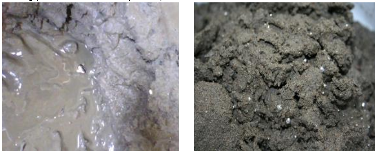
Figure 10. Fresh and dry tailings after a cyanidation leaching process. Mercury droplets can be seen in the tailings.
