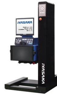
Fig.2 Appearance of headlight testing machine.
